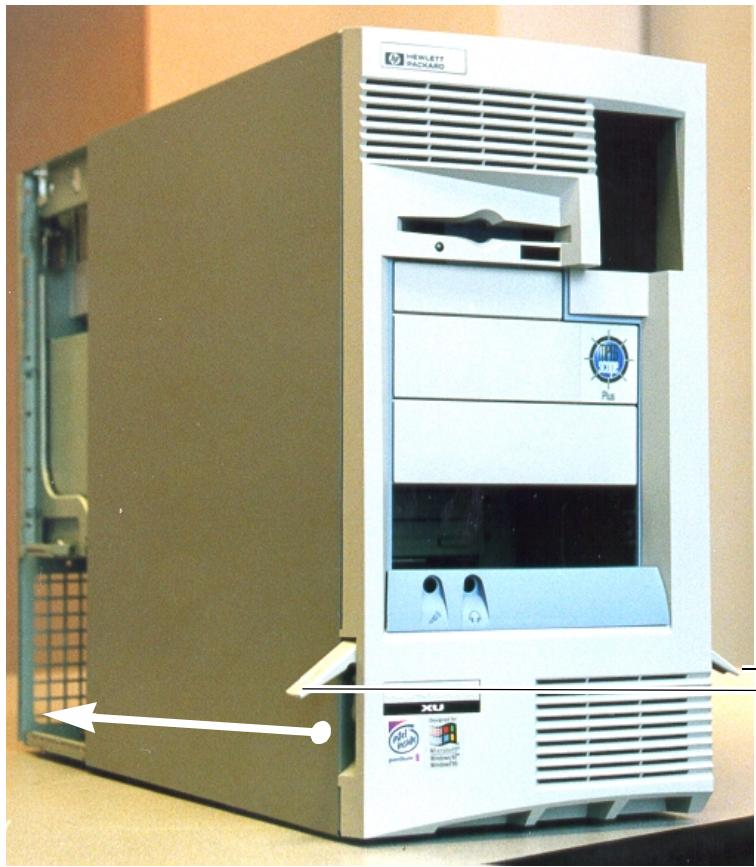
① Ensure that the two latches on the front sides of the cover are lifted up.
